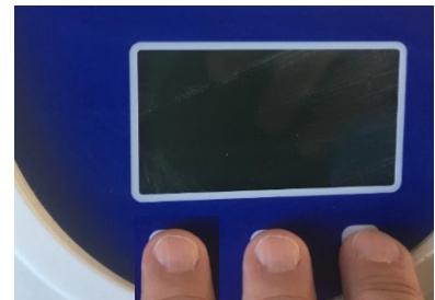
A successfully performed reset can be recognized by one short "beep"
