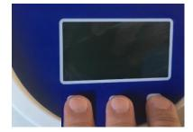
A successfully performed reset can be recognized by the fact that the operating hours on the start display are set to "0h".
