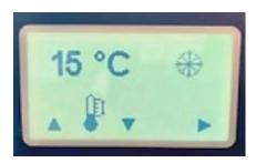
**Device is in operation** Device cools Pressure pump running
