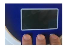
A successfully performed reset can be recognized by the fact that the operating hours on the start display are set to "0h".
